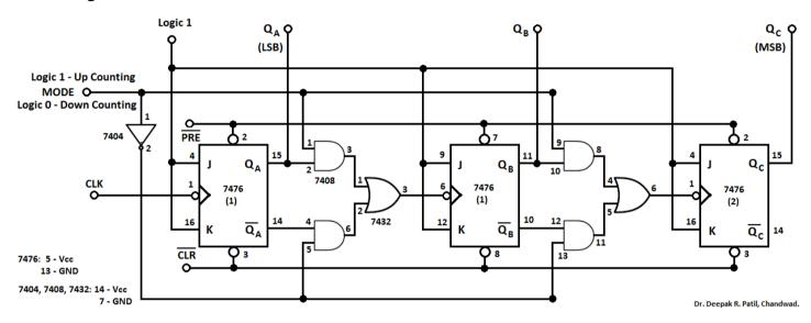
**Note:** Connect series combination of 220 $\Omega$  resistor and LED between output and ground to see output.
