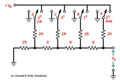
**Note: 1.** Use  $2R = 10k\Omega$  or any value and  $R = 5k\Omega$  can be obtained by connecting two 2R resistors in parallel.
