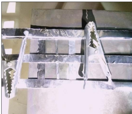
Fig 3 Masking on FTO for \text{TiO}_2 deposition
