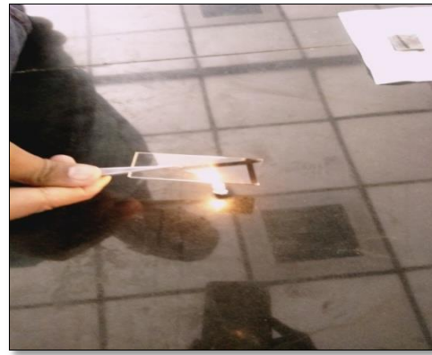
Fig. 6-b Graphite layer deposited on FTO
