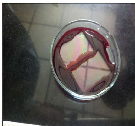
Fig. 5-b cell A and B are dipped into Beet
